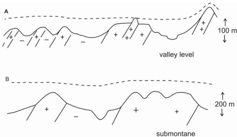
Fig. 2. Relation of two main levels and their preservation to lithology (rock resistance) in the flysch Carpathians; 1 — present-day relief (continuous line) and primary flat level (dashed line), + and — signs indicate various resistance of bedrock; levels: A — valley level (VL), B — submontane (SM)
